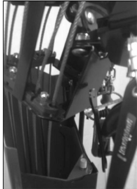
11. Check the cable routing to ensure that no tools are tangled. It is recommended that you pull on each tool to check for smooth operation.
