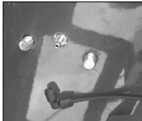
6. Connect the elbow to the pump outlet. You will now install the weight guard. Route the air line through the slot.
