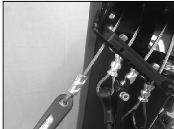
12. Tighten the large nut that secures the tool assembly carriage to the stand using a 19mm (3/4") wrench.
