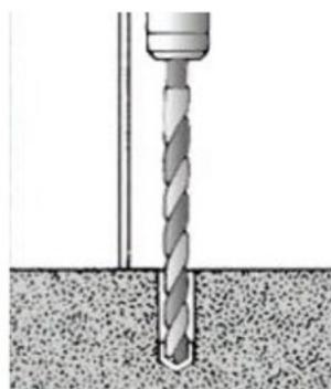
19. Before proceeding with installation, the hole must be cleaned of all concrete dust to ensure proper fastening. Use a wire brush, a vacuum or compressed air to clean out the hole completely.
