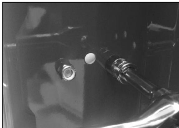
9. Install the plastic cover. Start by feeding the bottom edges of the cover into the side grooves at the top of the stand and slide it down. Be sure it is seated into the slot at the base.
